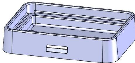
3. Place electronics board back into the base. Place buttons and snap lid back to base.
